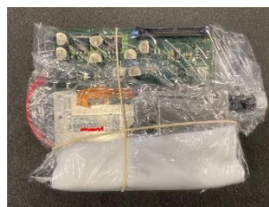
Seal the printhead with shrink wrap or place it inside a plastic bag
