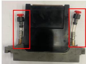
Without tubing : Use a Printhead Shut-off Kit.
