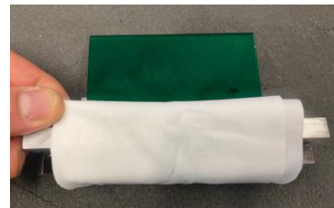
Fold the wipe around the printhead
