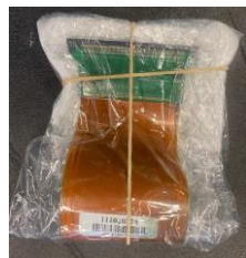
Seal the printhead with shrink wrap or place it inside a plastic bag
