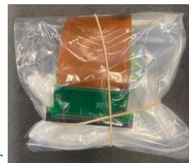
Seal the printhead with shrink wrap or place it inside a plastic bag
